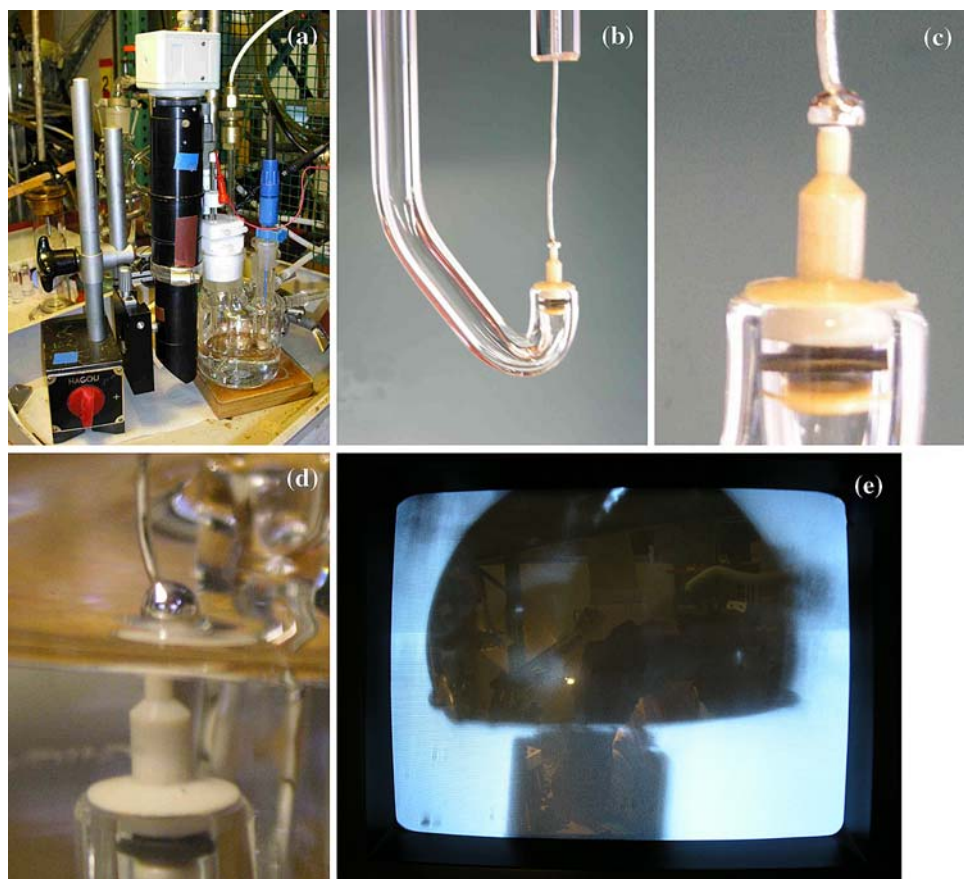
Fig. 2. Photographs of (a) electrochemical cell with the tip configuration and connection to the MS, (b) and (c) Tip – bead-type electrode configuration, (d) tip-electrode in hanging meniscus, (e) view of the tip-electrode configuration on the video screen.
